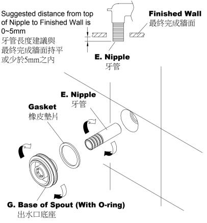
\* Apply the pipe compound or thread sealant tape and then screw it to the Valve Body. Suggested distance from top of Nipple to Finished Wall is 0~5mm, and Nipple could be cut if necessary. Screw the Base of Spout (With O-ring) with Gasket clockwise to the Nipple till against the Finished Wall. Please notice the Gasket has to be placed between base and wall.
