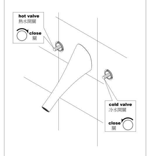
\* Turn hot and cold cartridge valve to closed position as aboved figure. 將冷熱水開關轉至關水位置,熱水開關順時鐘轉到底關閉,冷水開 關逆時鐘轉到底關閉。
