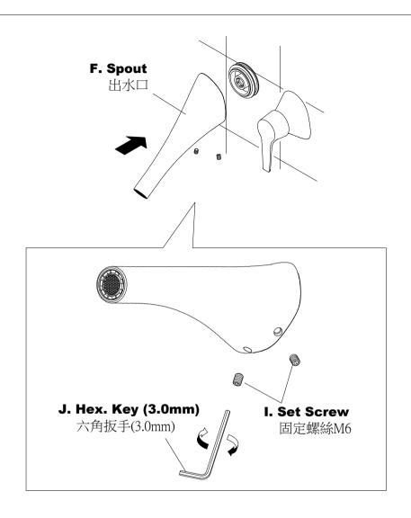
\* Position **Spout** onto **Base of Spout**, and then fix with provided **Set Screws** and **Hex Key**.
