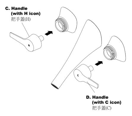
\* Confirm hot and cold valve have been turned to closed position before install the **Handles**. Press hot and cold **Handles** onto valve spindles until hear the click sound as the figure shows.
