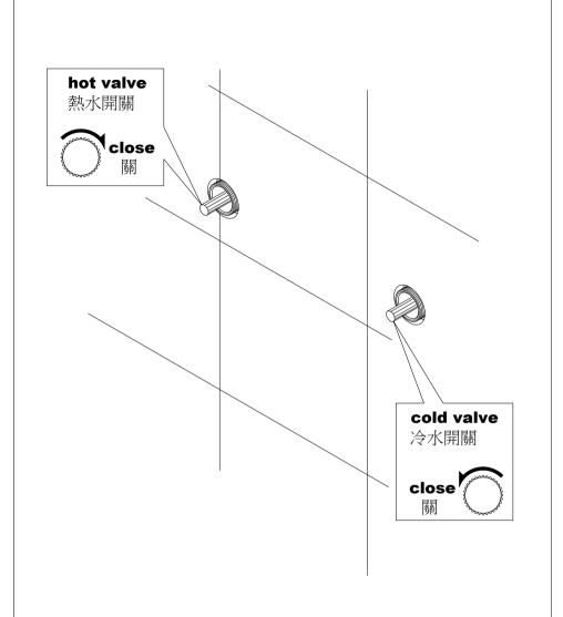
\* Turn hot and cold cartridge valve to closed position as aboved figure. 將冷熱水開關轉至關水位置,熱水開關順時鐘轉到底關閉,冷水開 關逆時鐘轉到底關閉。
