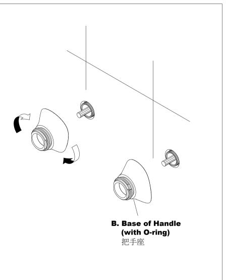
\* Screw the **Base of Handle** to the shanks of hot and cold valves till against finished wall.
